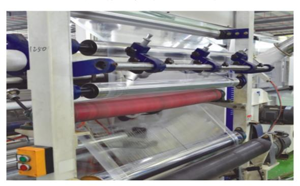
Automatic rewinding slitting device, high accuracy, reduce defective. 自動收卷分切裝置,準確性高,減低次品。
